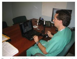
**Figure 2** The VisitOR1<sup>TM</sup> can be remotely operated with through a portable, laptop ControlStation that is linked via the Internet over a secure broadband connection.
